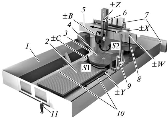
**Fig. 1.** VMG 50 machining center (with operator 11 to provide a sense of scale): (1) barrier; (2) milling table of blank (4.5 × 3 m); (3) gantry; (4) turning table (diameter 5 m, height 3 m); (5) gantry crossbar; (6) carriage; (7) control-system cabinets; (8) tool-replacement mechanism; (9) operator cabin with terminal and portable control panel; (10) guides for gantry.
