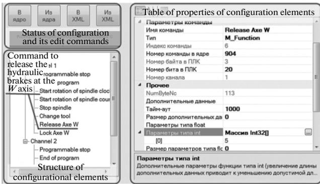
Fig. 5. Dialog screen for editing the command to release the hydraulic brakes at the  $W$  axis for the CNC-PLC interface.
