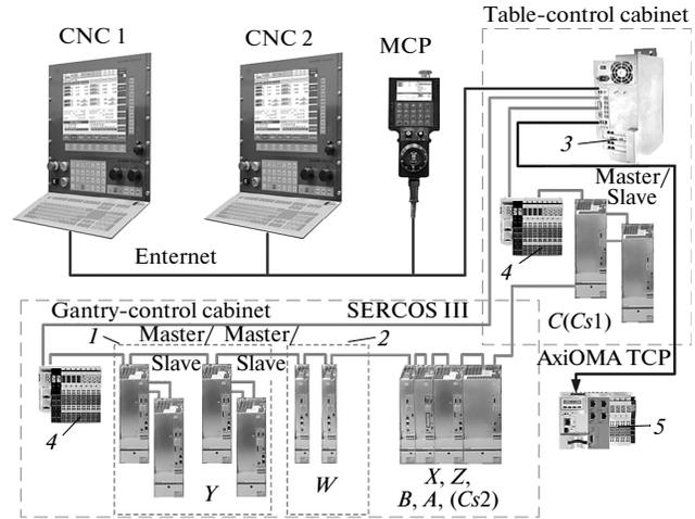
**Fig. 2.** Modular structure of the AxiOMA Contol CNC system for the VMG 50 machining center: MCP, manual control panel; (1, 2) gantries; (3) CNC kernel; (4) bus coupler; (5) controller of autonomous equipment.
