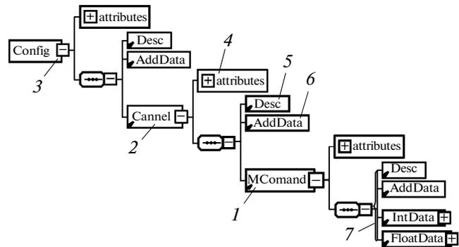
**Fig. 4.** Structure of the file data for the configuration of M commands at the CNC-PLC interface: (1-3) configurations of the M-command, the control channel for the command, and the CNC-PLC M commands, respectively; (4) attributes with data fields; (5) text description; (6) additional data set; (7) command parameters.
