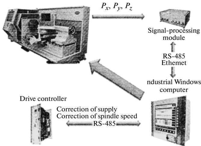
Fig. 3. Diagnostic system as an integrated component of a numerical control system.
