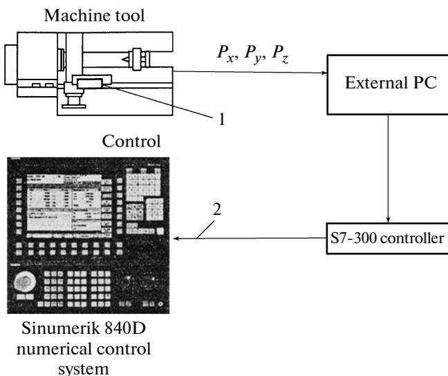
Fig. 4. Diagnostic system as an external module: (1) tensometric sensors; (2) correction of supply and spindle speed.
